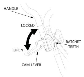
**FIGURE 12:** Adjusting The Height Of The Handle. (Lever shown in OPEN position)
