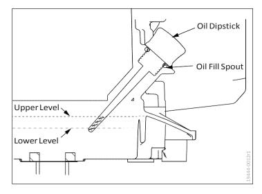
FIGURE 4: Filling Engine with Fuel and Oil.
