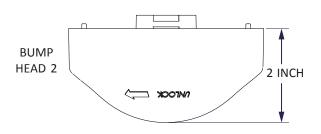
**FIGURE 13:** Setting The Height Of Your Cut With Bump Heads.
