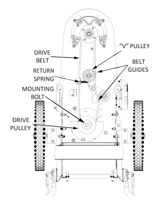
FIGURE 15: Routing The Drive Belt
