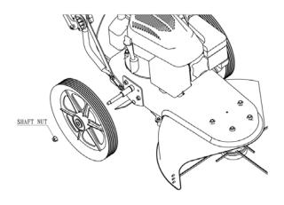
FIGURE 11: Removing the Wheels.
