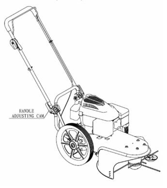
**FIGURE 3:** Adjusting the Handle Bars.
