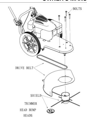
FIGURE 14: Mower Head Housing and Shield
