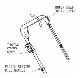
FIGURE 5: Using The Mower Head Drive Lever.
